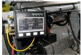
GPS tracks each car as it traverses the stage, and alerts HQ if a car is off- and where! Plus a button for "OK" from the affected team. It has a car-to-car Wi-Fi capability that alerts to a passing request. It
